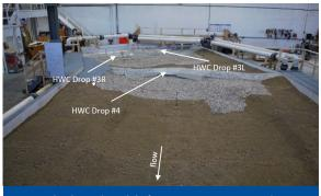
1:14 Scale Physical Model of HWC Drops #3L, #3R and #4
