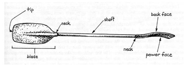
**Blade:** A kayak paddle has two blades attached at each end of a shaft. Each blade has two sides or faces. The side that is mainly used for pulling against the water is called the power face. The power face is slightly concave in shape, which helps hold water for greater resistance to pull against. The back of the blade is known as the backface. The backface tends to be slightly convex. The ends of the blade are called the tips.
